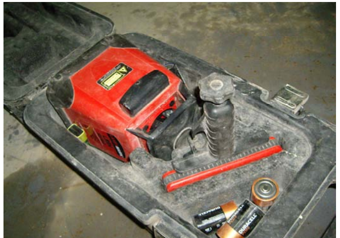
AUTOLIVELLO LASERMARK LMH SERIES
