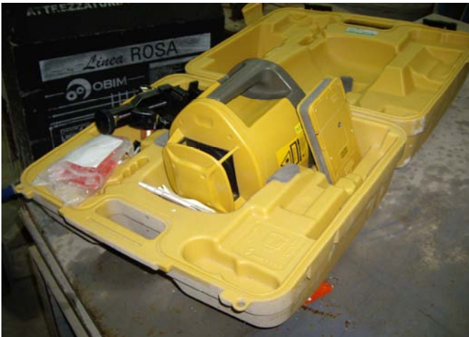
AUTOLIVELLO LASER TOPCON RL-H3C
